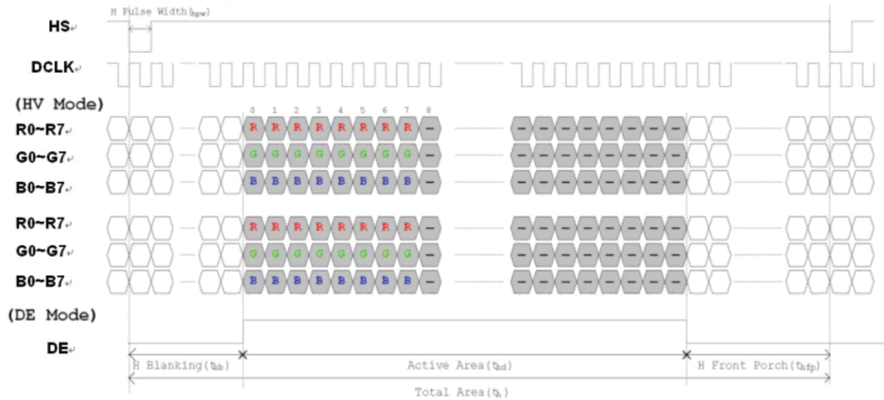
Figure 5: Horizontal Input Timing Diagram
